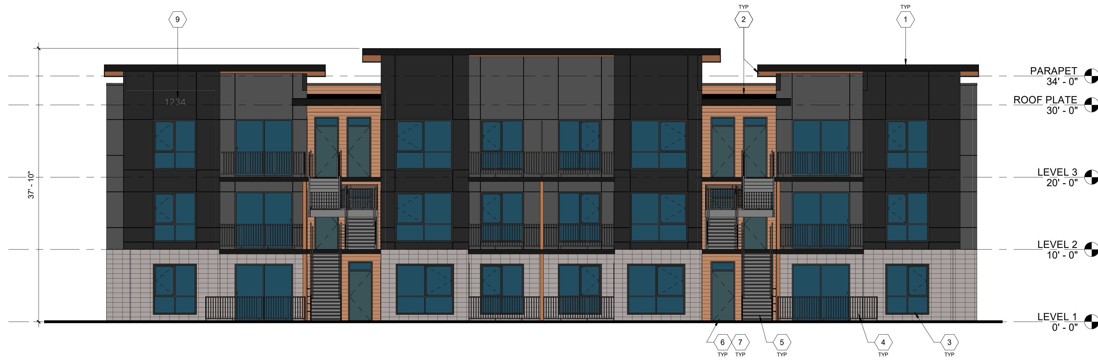
1 BUILDING B1- BUILDINGS #4, #5, #6, #12, #15 - FRONT ELEVATION
