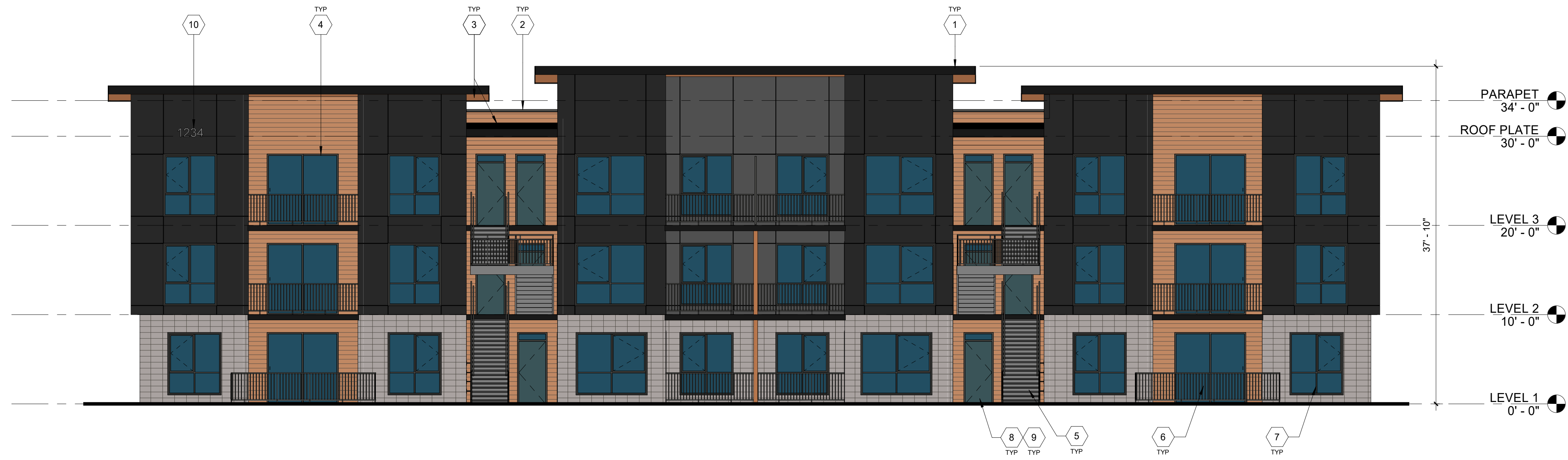
1 BUILDING B3 - BUILDING #9 - FRONT ELEVATION 1/8" = 1'-0" @ FULL SIZE
