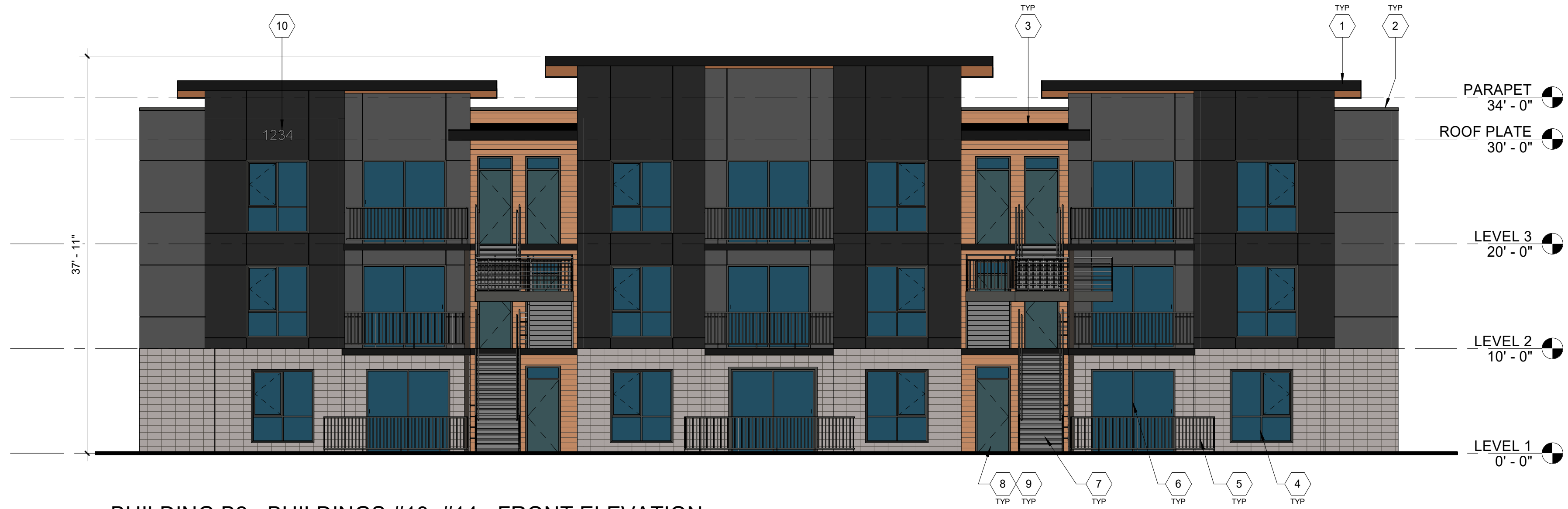
1 BUILDING B2 - BUILDINGS #13, #14 - FRONT ELEVATION 1/8" = 1'-0" @ FULL SIZE
