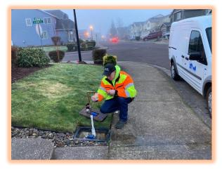
Water Technician collecting a water sample for testing.
