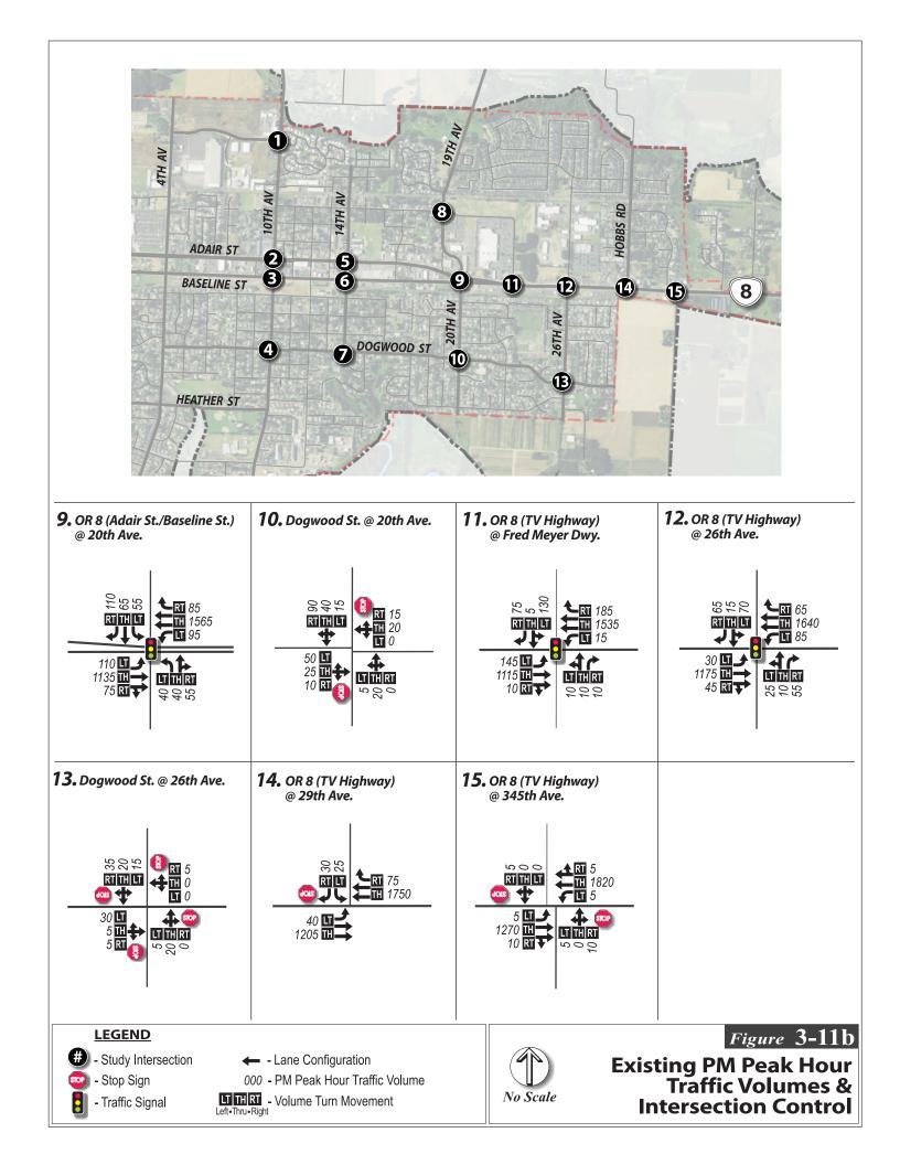
The PM peak hour intersection counts were used to determine the existing level of service based on the 2000 and 2010 Highway Capacity Manual methodology<sup>13</sup>. Traffic counts and level of service calculation sheets will be provided in the TSP appendix. Table 3-6 summarizes the existing weekday PM peak hour study intersection operation conditions.
