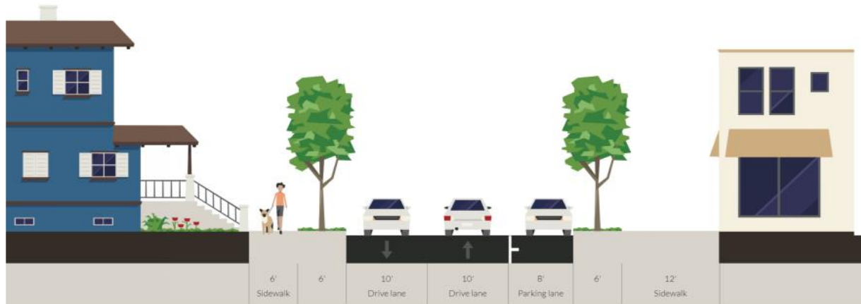
Figure 3. 14 th Avenue Greenway Cross-section
